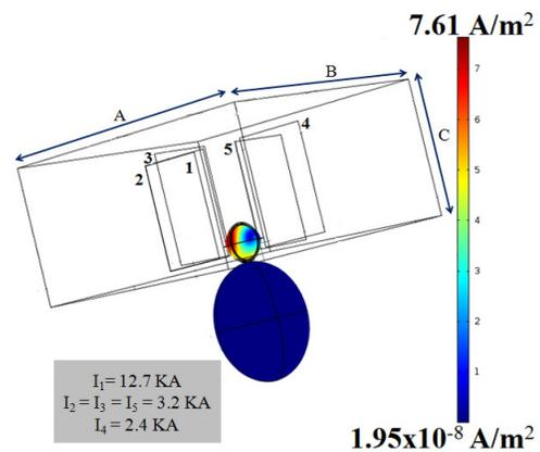
Figure 5. Three-dimensional view and main characteristics of the optimized orthogonal configuration studied here. The number of coils, their current values (termed I<sub>1</sub>-I<sub>5</sub>), together with the minimum and maximum values of current density achieved are shown.
