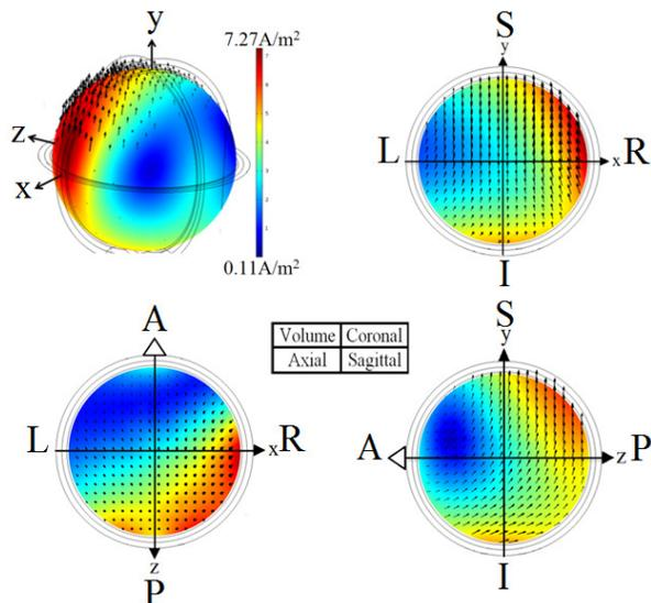
Figure 7. Current density distributions for the optimized orthogonal configuration stimulating mainly the right hemisphere, which could be further tilted upon need. The coils and part of the head sphere are immersed in conducting liquid.
